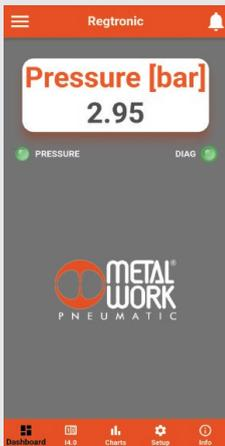
The Metal Work RegUp App can be used for connection via Bluetooth to Metal Work proportional pressure regulators in the REGTRONIC series with a wireless interface, from Android smartphone and iOS.
