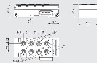
\* Connectors usable also for reading direct current motor encoders
