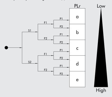
If, for example, the severity of a lesion resulting from a failure is low and/or the hazard exposure frequency is low and/or the hazard avoidance possibility is high, the PLr will be low. On the contrary, if the severity and/or exposure frequency is/are high and/or the hazard avoidance possibility is low, then the PLr for that safety function will be high.
