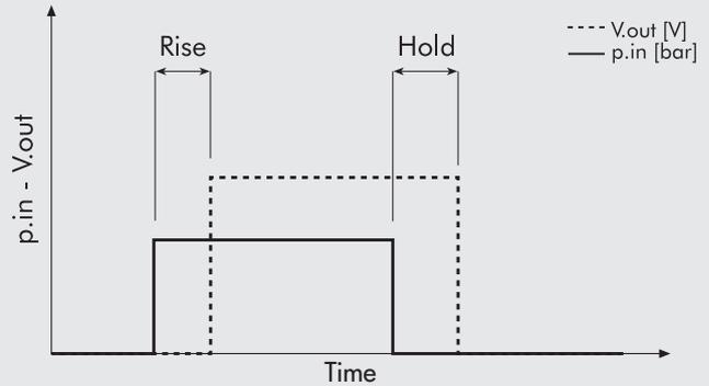
**Rise time:** the delay from activation of the compressed air supply to 24V power supply to the M8 connector.
